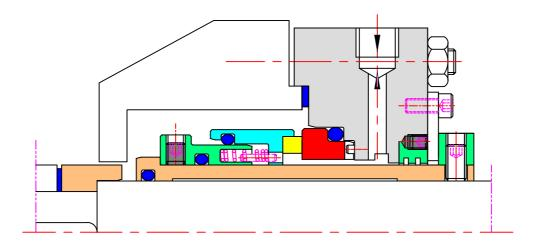
90 SERIES MULTI SPRINGS MECHANICAL SEAL TYPE 9302 CARTRIDGE ARRANGEMENT WITH DIFFERENT API PLAN 62
